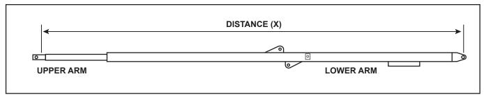
d. Pin the Arm Extension Cylinder in position on the arm and use this to determine the location of the upper arm mounting plates. **NOTE:** Be sure the cylinder piston is fully seated.
