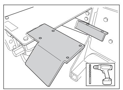
j. Mount the Spool Valve and PriorityFlow Valve to the new brackets.1/4" bolts and nuts recommended.
