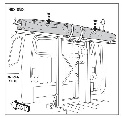
**NOTE:** Visually align the torsion axle with the center of the gantry front to back.
