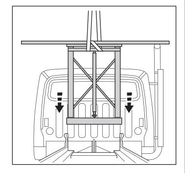
IMPORTANT: Check all position measurements to be sure gantry is centered, square with frame and proper clearances are all accounted for.
