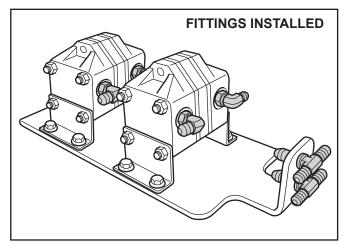
d. Mount the bracket with valves in position at the cross member. Be sure to maintain proper clearance.
