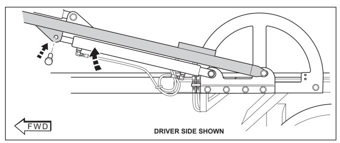
i. Install upper pivot of the Arm Extend/Retract cylinder with 1/2" x 2" Clevis Pin.
