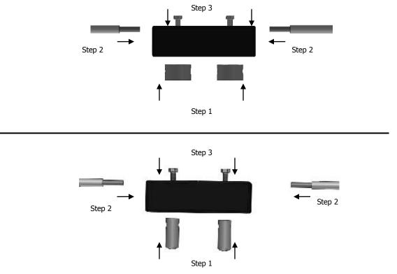
Mount the angle iron by bolting or welding in place. Attach assembled poly blocks to the angle iron as shown below. Note on the side with the springs, only run the nut on until there are 2 threads sticking through the nylock in the nut. **Make sure the wires will not interfere with any thing that may chaff or pinch them.**
