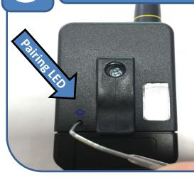
Place GTX Transmitter in Pairing Mode
